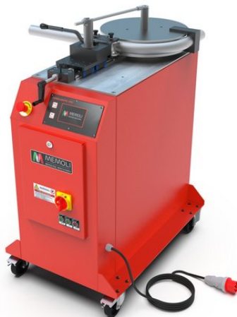
With device AB-CT for tube bending without mandrel
