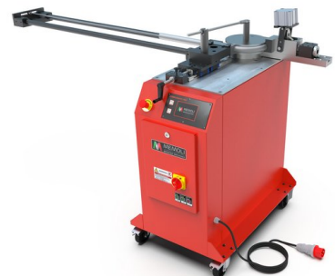
With device AB-CTA for tube bending with mandrel and pneumatic vice
