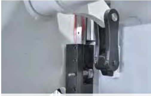
Hassas Büküm sağlayan dengeleme kolu Torsion bar enabling sensitive bending
