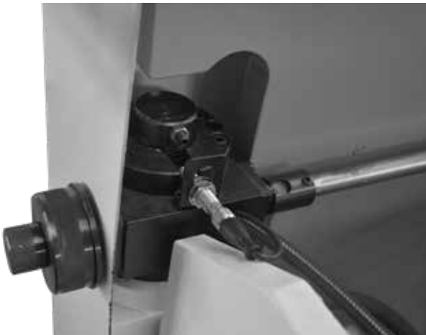
Model EB 1230 NC & MOTOR Kontrollü Y Eksen (Açı Ayarı) Model EB 1230 NC & MOTOR Controlled Y Axis (Angle Set Adjustment)
