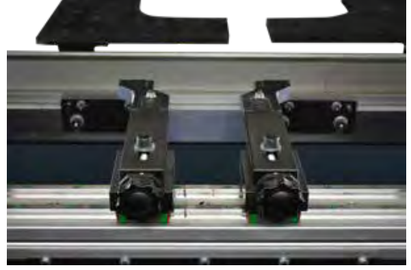
Motorlu Arka Dayama Motorized Backgauge
