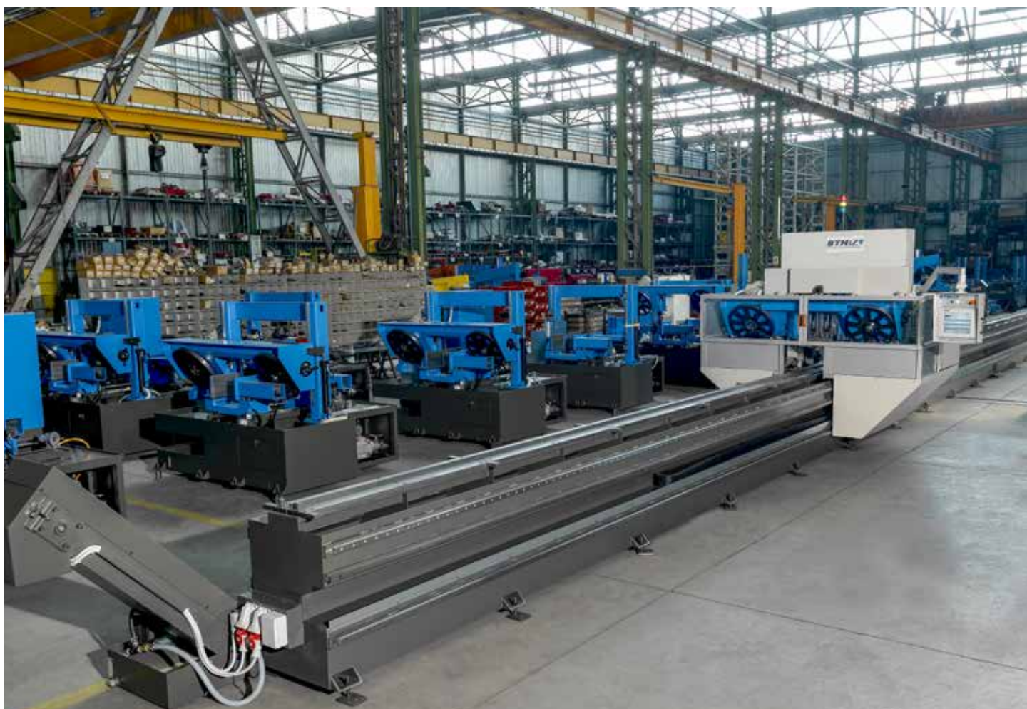
Impianto speciale per taglio e foratura binari con diametro massimo 40 mm Special system for cutting and drilling tracks with a maximum diameter of 40 mm
