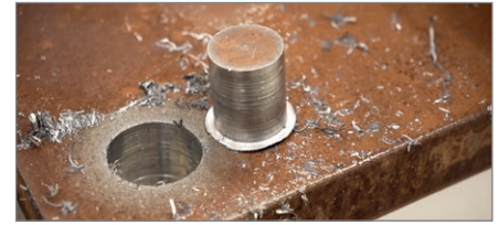
Max milling capacity up 40 mm (1-9/16")
