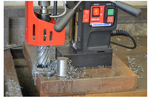
Milling capacity up to 50 mm (2") Depth of cut up to 75 mm (3") - option
