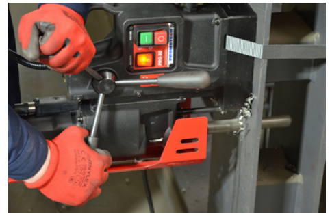
Drilling capacity up to 23 mm (0.91")
