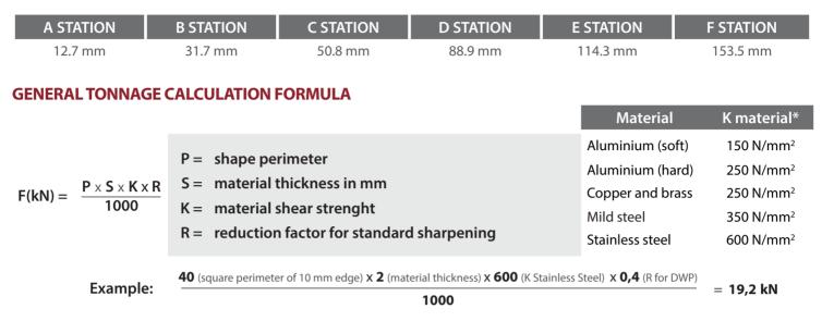
\* The table shows average coefficients for standard sheet metal. For a specific tonnage calculation it is necessary to know the exact characteristics of the material.
