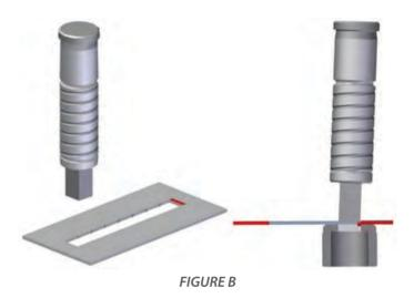
On such situation, due to side load, the tool tendes to lean over the sheet, causing the following:
