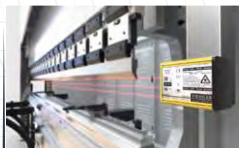
CE Laser Safety System
