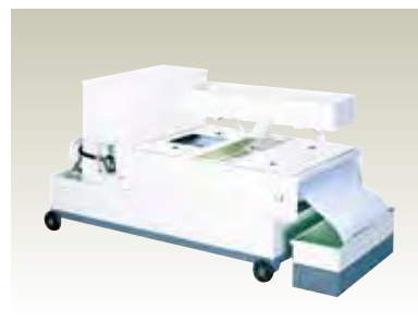
COOLANT SYSTEM WITH AUTO PAPER FEEDING DEVICE (With 1 Roll of Paper) B17-0301 Volume: 120L Paper feeding motor: 25W Pump: 1/8HP Coolant Capacity: 20L/min Space: 57"x24 3/8" (1450x620mm) Height: 30"(760mm)
