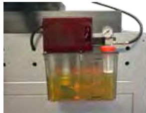
Otomatik Malafa Yağlama (Opsiyon) Automatic Mandrel Lubrication (Optional)
