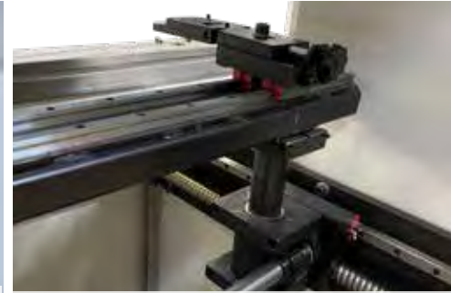
Motorlu Vidalı Mil Arka Dayama Motorized Backgauge with Ballscrew
