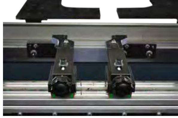
Motorlu Arka Dayama Motorized Backgauge
