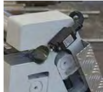
Standart kafa açma vıçı Standard drop-end safety switch
