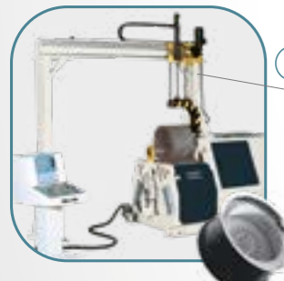
Hydraulic Automatic Wheel Rim Body Production Machine and Hydraulic Plate Ejector. Mass production cycles
