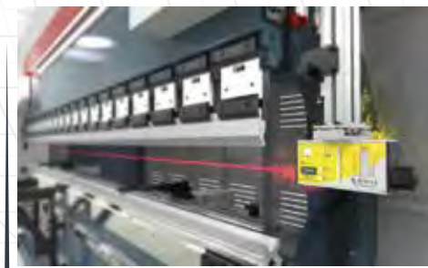
CE Laser Safety System
