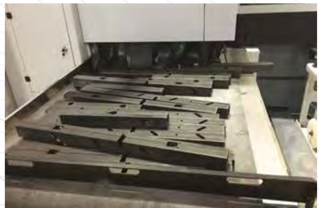
Tubes up to 6 m of length are removed by automatic unloading system with conveyor.
