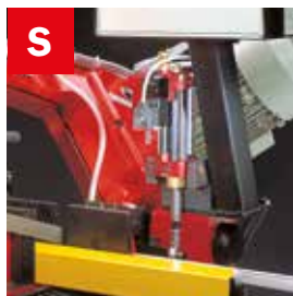
S SKIP ELETTRICO Electrical skip
