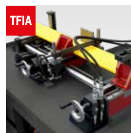
TFIA TAGLIO FASCIO OLEODINAMICO Hydraulic bundle clamping device
